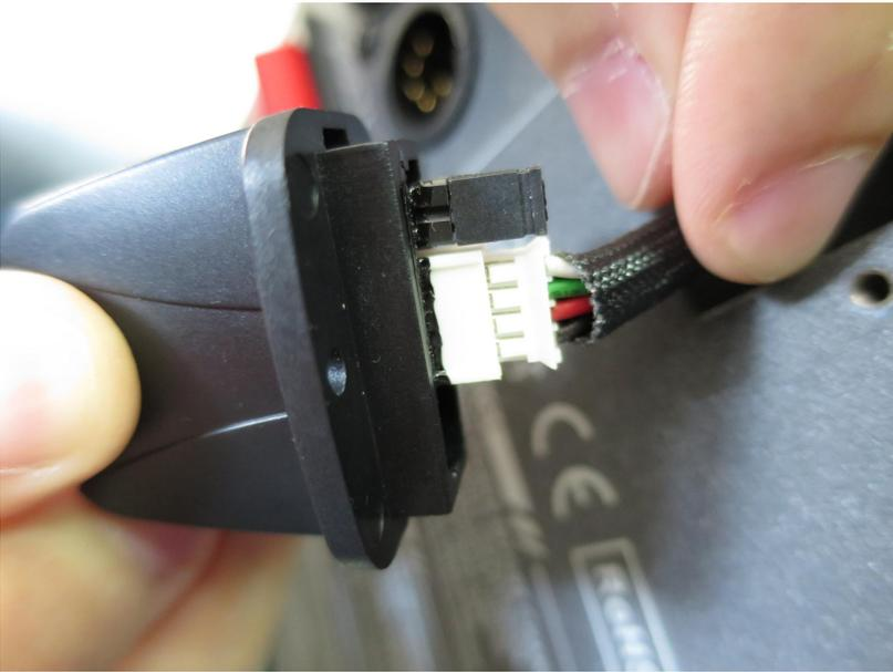
Step 4: Screw the receiver on machine tightly.
