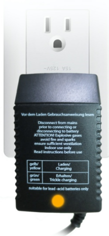
Yellow indicates charging
