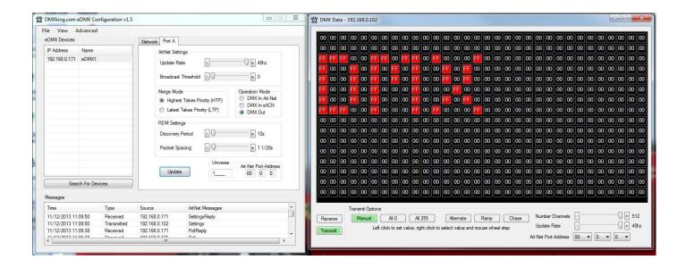
Changing to Receive mode will display the selected Art-Net universe number with merged streams if more than 1 is present. Note Art-Net II unicast is not supported meaning only Art-Net broadcast streams are displayed.
