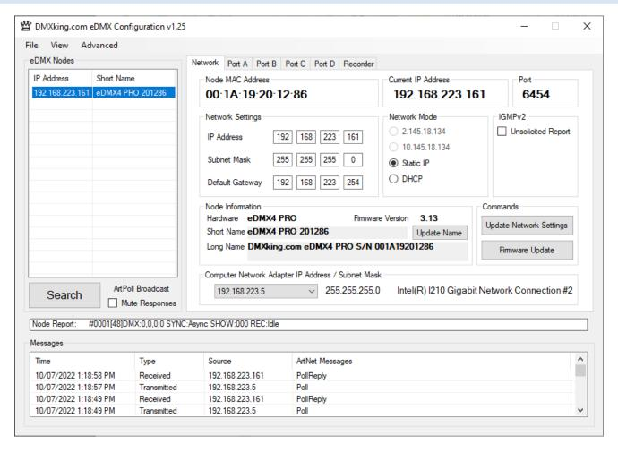
Before starting the eDMX Configuration utility please ensure your computer has appropriate IPv4 network settings, for example IP 192.168.0.100 Subnet 255.255.255.0 Gateway 192.168.0.254.
